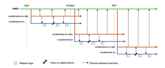
EWAOL's branch and release process is based on the Yocto release process. The following sub-sections describe in more details the branch strategy for EWAOL's development and release process.
