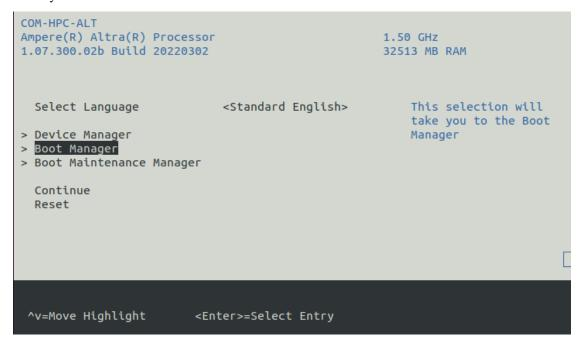
15. **On the Serial Console Terminal:** the connected USB storage device containing the AVA Flasher Image should then be visible in the Boot Manager Menu. Highlight that USB storage device entry using the arrow keys and select it by pressing the ENTER key. An example Boot Manager Menu showing a connected USB storage device is shown in the following image:
